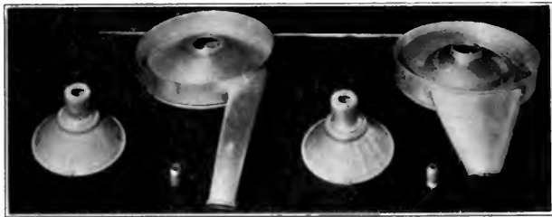
FIG. 2.—LEFT, BOWL PARTS USED FOR SEPARATING NORMAL CREAMS; RIGHT, THOSE FOR SEPARATING HIGH-TESTING CREAMS, FACTORY-SIZE SEPARATOR
